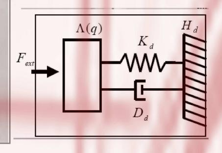
By using VIAs, the natural oscillatory dynamics of the system can be tuned to closely resemble the desired periodic motions required for the gait patterns. In addition, introducing compliance to the legs can enlarge the intrinsic overall robustness of the system to disturbances.
