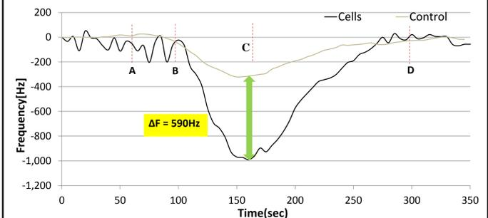
Figure 7. Frequency output of a dual SAW sensor in response to the introduction of 12.5 μM octopamine. The *Sf9* cell-coated sensor's response is shown in black, the uncoated reference sensor's in grey.
