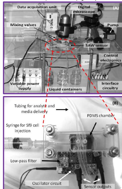
Figure 5. Photograph of the computer-controlled microfluidic system, sensor drive and interface circuitry (A) with an assembled dual SAW biosensor with its associated oscillator circuitry (B).
