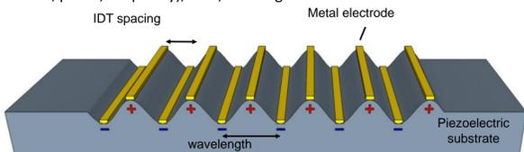
Figure 2. The basic principle of exciting surface acoustic waves by an interdigital transducer created by micro-patterned metal electrodes on a piezoelectric substrate
