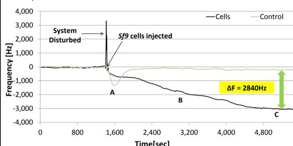
Figure 6. Frequency output of a dual SAW sensor in response to deposition and adherence of *Sf9* cells on the sensing sensor surface.
