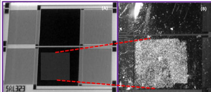
Figure 3. Optical micrograph of a metalized dual SAW biosensor (A) and the same biosensor functionalized with adherent *Sf9* cells (B).
