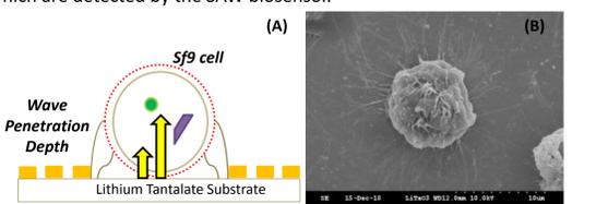
Figure 4. Schematic representation of a *Sf9* insect cells on a LiTaO<sub>3</sub> SAW microsensor with the associated acoustic wave penetration depths (A) and the scanning electron micrograph of a *Sf9* cell adhered to the surface of a LiTaO<sub>3</sub> SAW device after 1hr (B).
