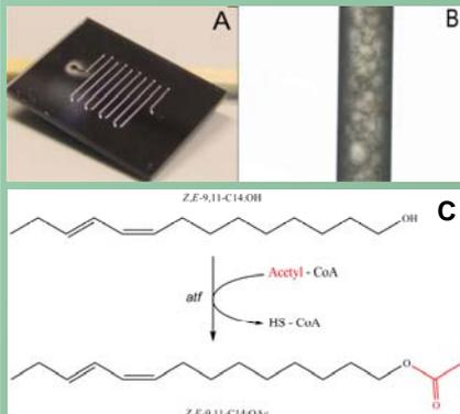
Figure 1. Biomicroreactor: A) Glass-silicon microreactor, meander channel with rectangular cross-section (0.25 x 0.20 x 91.26 mm); B) Agarose beads (Novagen) inside the microchannel; C) Pheromone biosynthetic reaction
