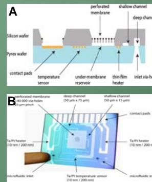
Figure 2. Evaporator: A) Schematic representation of the evaporator chip cross-section; B) Image of the evaporator, channel side visible
