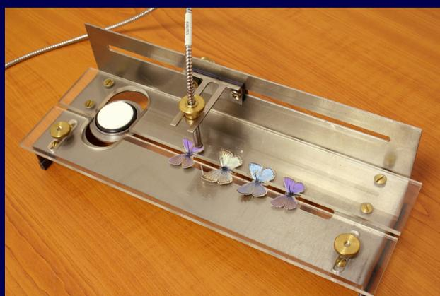
Figure 4. "Spectroboard" in use. Prepared specimens can be measured rapidly and safely in reproducible conditions.
