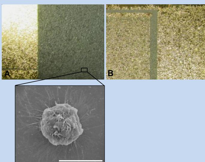
**Figure 3.** Sf9 cell adherence to varying SAW device surfaces. Sf9 cells adhere, within 1hr, to both LiTaO<sub>3</sub> (A) and gold (B) SAW device surfaces. Images were captured using a stereo microscope at 50x magnification. Inset image - scanning electron microscopy of an Sf9 cell adhered to the surface of a LiTaO<sub>3</sub> SAW device after 1 hr. Scale bar 10µm.
